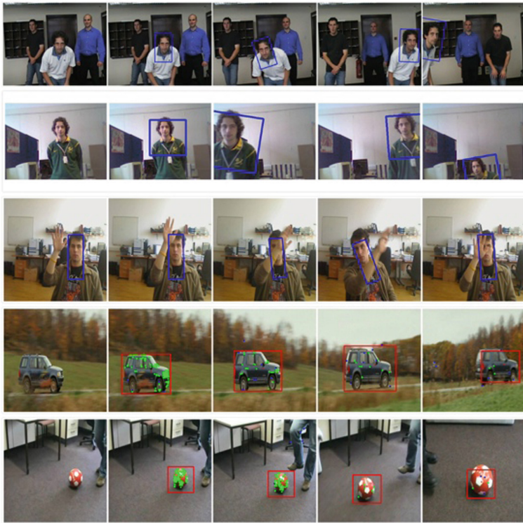
Fig. 2. The experiments on different type of objects show that rigid objects with more corner features will have better tracking performance.
